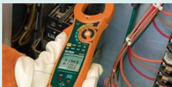
2.0" (52mm) jaw size for conductors up to 500MCM
