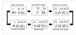
Stopwatch with 6 modes: Time/Date, Heat Index, Chrono Lap, Alarm, Timer, and Chrono Split Mode
