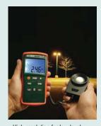
High resolution for low level measurements in places like parking lots, stairwells, and ATM machines
