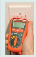
Built-in Non-Contact Voltage Detector. Red LED bar lights when live wire detected.
