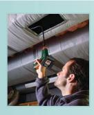
Extech Borescope features a 2.25" color monitor with video output for viewing on any monitor and a waterproof 9mm camera with bright LED lights.
