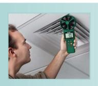
Extech's 4" (10cm) Large Vane Thermo-Anemometer series allows for more precise readings on larger size ducts. Each meter simultaneously displays Airflow or Air Velocity and Temperature. Choose models that also measure Air Volume, Humidity & Carbon Dioxide (CO2).
