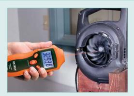
Non-contact fan blade RPM or REV testing
