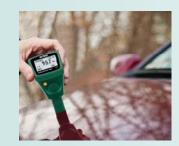
Extech's CG304 offers a non-destructive way of measuring the thickness of ferrous and non-ferrous substrates with auto recognition of the material being measured. Unique Bluetooth interface feature wirelessly transmits measurement data to your PC for further analysis and to generate a documented report.
