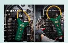
Flexible 11" (28cm) clamp jaw easily wraps around bus bars and cable bundles that may be difficult to access with regular clamp meters. The thin 8mm cable diameter easily fits into tight spaces. Includes test leads for multimeter functions measuring Voltage, Resistance, and Capacitance. True RMS and CAT IV rated allows for maximum accuracy and safety for your measurements.
