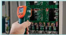
Detect hot spots on circuit breaker panels
