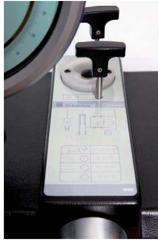
Control schematic on the CPB3800HP instrument base
