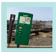
Compact handheld Conductivity Meter with long life carbon rod combination electrode measures Conductivity, TDS and Temperature. Units of measure include  $\mu\text{S/cm}$ , mS/cm, ppm, °F, and °C. The meter features three ranges for Conductivity and TDS plus adjustable Temperature compensation factor to maintain accuracy.
