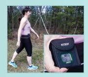
Extech's pocket-size Pedometer offers 3D Sensor design for detecting motion regardless of orientation, plus it measures Temperature! The fully-loaded PD20 has many other functions including Step Counter, Timer, Distance meter, Speedometer, Calorie Counter, Fat-Burning meter, and Storage Memory. It includes a protective case and can clip onto clothing or can be worn around the neck (lanyard not included); also fits easily into a pocket or purse.
