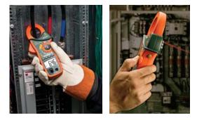
CAT IV -600V safety rating for added protection and True RMS feature gives you accurate readings of non-sinusoidal waveforms. Built-in IR Thermometer with laser pointer is an excellent troubleshooter for locating hot spots and overheating motors.
