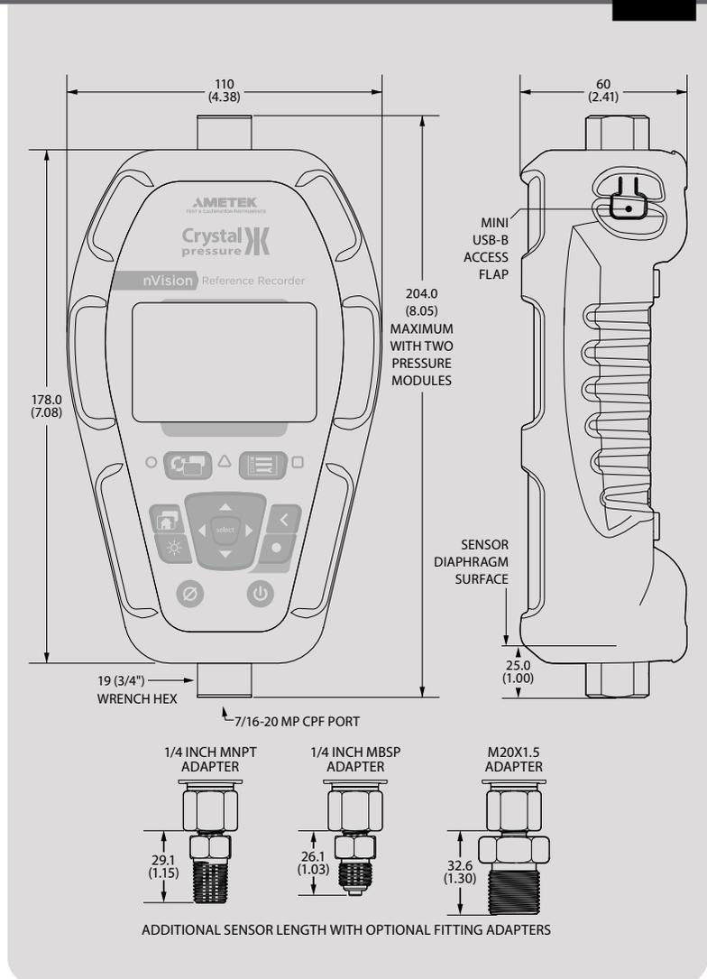
ADDITIONAL SENSOR LENGTH WITH OPTIONAL FITTING ADAPTERS
