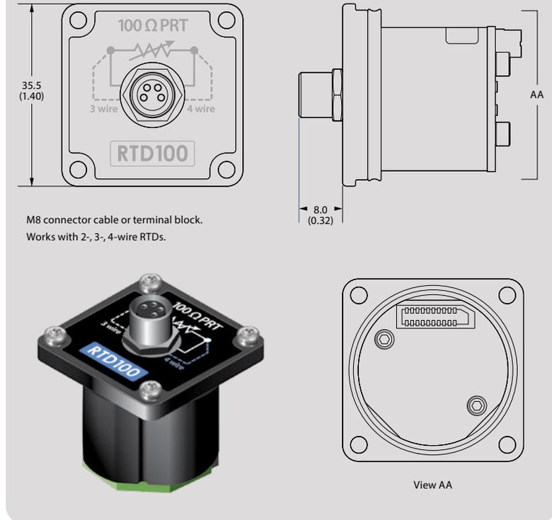
M8 connector cable or terminal block.
