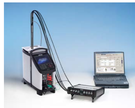
An ASM-803 A connected to the inputs of a JOFRA RTC calibrator, and controlled by JOFRA-CAL.
