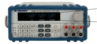
The 9130 is a fully programmable triple Output DC Power Supply delivering 0-30V/0-3A on 2 outputs and 0-5V/0-3A on 1 output. Each output is fully floating and outputs can be adjusted independently or connected in series or parallel to produce higher voltages or currents. The 9130 is ideally suited for applications in Electronic Test, Production and Service where multiple independent DC supplies are required and bench space is at a premium.
