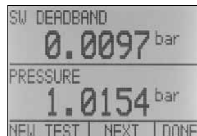
Quasi automatic pressure switch test, records automatically, open, close and deadband values
