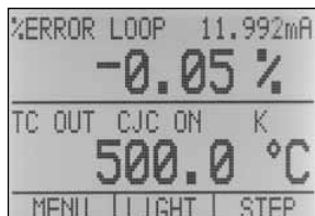
Online % error calculation, fast and responsive reading, for calibration and adjustment tasks
