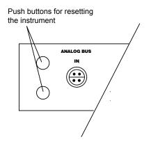
The push buttons on the back of the B-models can only be used to reset the instrument.
