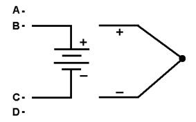
See section 10.0; Technical specifications for supported types of thermocouples. The multi-scanner has a cold junction compensation function. Normally this function should be ON and the actual temperature of the thermocouple can be measured. With CJC OFF, the multi-scanner will measure the difference between the thermocouple at the junction and at its TC input terminal.
