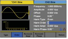
Generate harmonics up to the 10th order with independent amplitude and phase settings.
