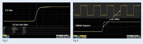
Generate high performance square waves with < 3.4 ns rise/fall times (Fig 5) and rms jitter < 300ps + 0.05 ppm of period (Fig 6)
