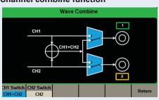
Create complex waveforms by internally adding each channel's waveform and outputting the combined waveform on channel I or 2.
