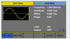
Save time with the 4050B Series' two independent channels to output synchronous signals. With a push of a button, all waveform parameters can be quickly copied between channels to set up identical output signals. Phase between channels can also be adjusted from the front panel.
