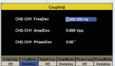
Customize your generator's channel output configuration with frequency, amplitude, and phase coupling. When enabled, CHI and CH2 can automatically track according to the user's set frequency, amplitude, and phase deviation ratio between channels.
