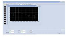
The provided waveform editing software can be used to create point-by-point arbitrary waveforms via freehand or waveform math functions. A standard USB interface on the rear panel allows users to easily interface with a PC to load these arbitrary waveforms into the instrument.
