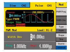
These instruments are capable of many different types of modulation for various applications. Modulate your waveforms with AM, DSB-AM, FM, PM, ASK, FSK, and PWM modulation schemes.
