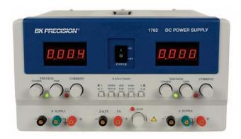
The 1760A series triple output DC power supplies offer three independent outputs with coarse and fine adjustment knobs for volts. The 4-digit LED display offers 10 mV and 1 mA resolution, providing the capability to set voltage and current values more accurately than 3-digit displays found in most comparable power supplies.
