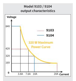
Traditional power supplies with rectangular output characteristics are only able to deliver maximum output power at one voltage/current point. The 9103 and 9104 provide greater flexibility over traditional power supplies by extending the operating areas. For example, the 9103 can operate at 42V / 7.6 A, 16 V / 20 A, or any other point on the maximum power curve.
