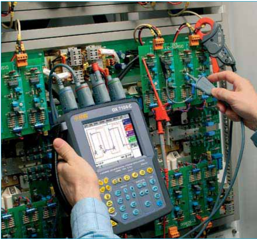
Field testing is quick and easy thanks to the Model OX 7104-C's hand strap and the use of PROBIX Smart Probes, some that have control buttons, with user definable functions, right on the probes themselves.
