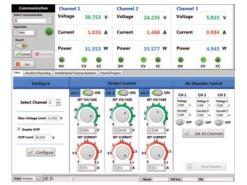
PC software is provided for front panel emulation, generating and executing test sequences or logging measurement data without the need to write source code.
