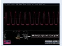
For applications requiring high signal integrity and edge stability, the 4060 Series can generate pulses with a low cycle-to-cycle jitter of < 100 ps.
