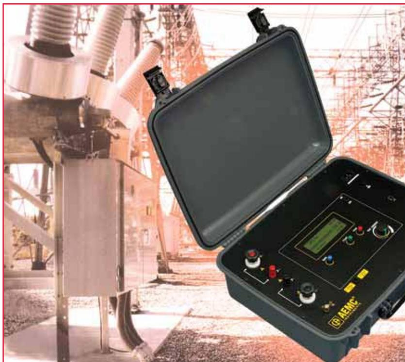
The AEMC® high-current Micro-Ohmmeter Model 6290 is a portable, microprocessor-controlled instrument. It has optimized filters and protection for measurements in electrical substation. The Model 6290 can be used to accurately measure very low contact resistances on high voltage circuit breakers, switches, busbars, etc., with test currents up to 200A. It employs the four-terminal Kelvin method to prevent errors caused by test leads and their contact resistances.
