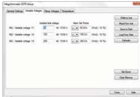
Variable Voltage selections from 40 to 5100V and can also be programmed along with alarm set points.
