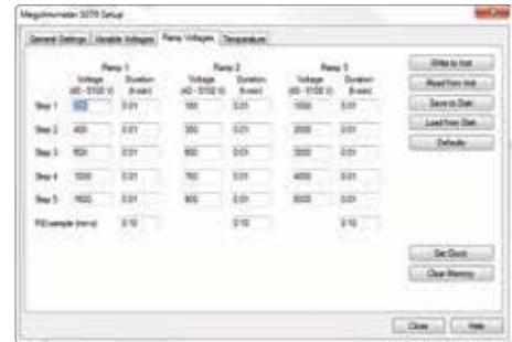
Model 5070 includes Ramp Function which allows programming of three different ramp test profiles, each containing up to five voltage steps between 40 and 5100V and time per step of up to 10 hours.
