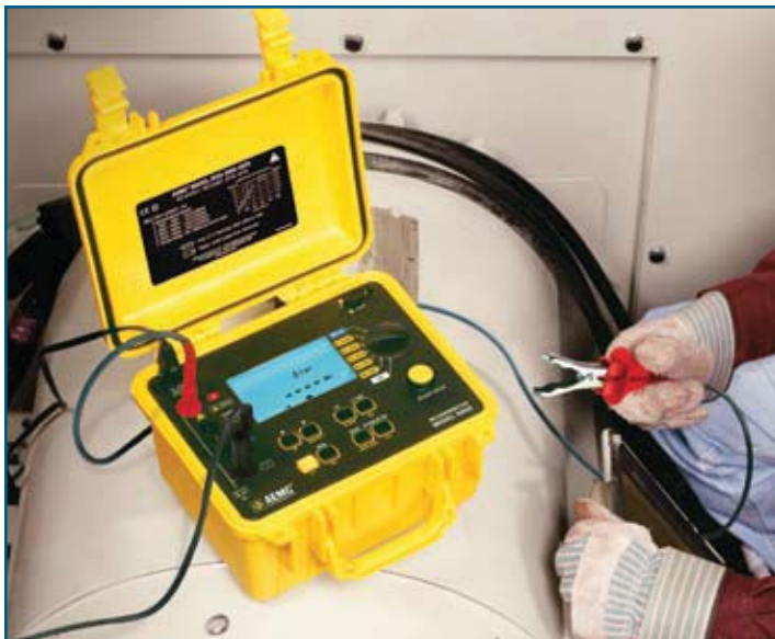
Model 5060 performing insulation test on a generator.
