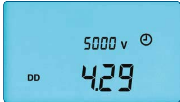
Automatic calculation and display of DD Ratio on request the conclusion of the test.
