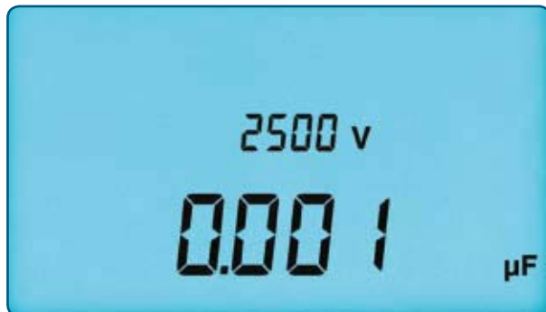
Capacitance Measurement from 1nF to 50μF displayed at the conclusion of each test.
