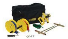
Test Kit for 3-Point testing includes two 150 ft color-coded leads on spools (red and blue), one 30 ft lead (green), two 14.5" T-shaped auxiliary ground electrodes, one set of five spaded lugs, 100 ft tape measurer and carrying bag.
