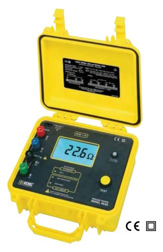
Digital Ground Resistance Tester Models 4620 and 4630 perform both ground resistance and soil resistivity tests. These testers measure from 0 to  $2000\Omega$ , and are auto- ranging, so they automatically seek out the optimum measurement range. Easy-to-use: simply connect the leads, press-to-measure and read the results.
