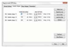
Variable Voltage selections from 40 to 5100V and can also be programmed along with alarm set points.
