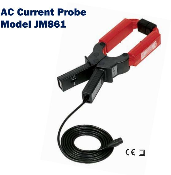
The Model JM861 is a high performance AC current probe for higher currents. Excellent transformation and low phase shift, plus a broad frequency response, permit accurate measurements of current and power. The high quality magnetic core and uniform windings provide for accurate measurements up to 3000Aac. The "squared" jaw permits multiple conductor or bus bar positioning. The Model JM861 provides excellent True RMS capabilities and reliable signal reproduction.
