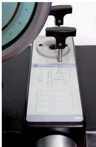
Control schematic on the CPB3800 instrument base
