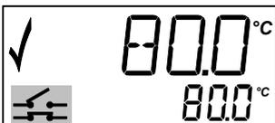
The calibrator will now start working towards the  $T_{\max}$  using the slope rate selected in SETUP. The flashing SWITCH TEST symbol indicates the current status:
