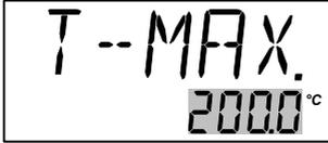
If the current set-temperature is higher than the new max-temperature, you will need to adjust the set-temperature. The instrument will immediately begin to cool (if required) as soon as the new max-temperature is accepted.
