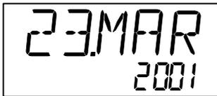
The calibration date will be displayed for approx. 2 seconds. The initialisation process has been completed and the calibrator is ready for use.
