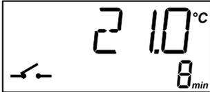
When the calibrator is stable the display will show the
