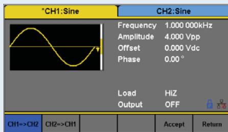
Save time with the 4050B Series' two independent channels to output synchronous signals. With a push of a button, all waveform parameters can be quickly copied between channels to set up identical output signals. Phase between channels can also be adjusted from the front panel.
