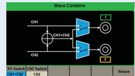
Create complex waveforms by internally adding each channel's waveform and outputting the combined waveform on channel 1 or 2.
