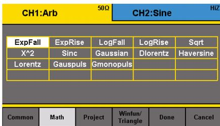
All models in the 4060 series provide non-volatile memory to create, store, and recall up to 24 different 16-kpt arbitrary waveforms and up to 8 different 512-kpt arbitrary waveforms. Users can also output any of the 36 built-in predefined arbitrary waveforms.
