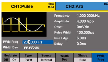
These instruments are capable of many different types of modulation for various applications. Modulate your waveforms with AM, DSB-AM, FM, PM, ASK, FSK, and PWM modulation schemes.
