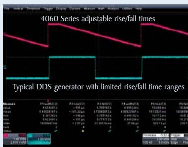
Capable of setting edge times within a large range, the 4060 Series can generate pulses with minimum rise/fall times of 6 ns and maximum rise/fall times of 6 seconds.
