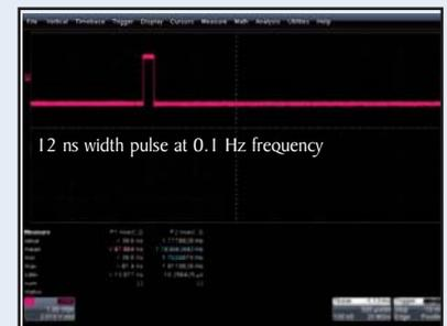
Unlike traditional DDS generators, the 4060 Series has the capability to output a rapid pulse at very low frequencies. Duty cycle can be set to as low as 0.0001%.
